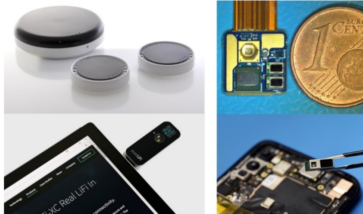
Fig. 4.2: Current commercial OWC transceivers (left) and their evolution toward miniaturized light antennas (right).
